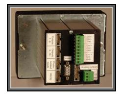
The three analog inputs, each assignable to any control channel, connect directly to the analog input terminal board.
